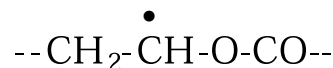
Scheme 3. The proposed chemical structure for the secondary alkylether radicals created in PCL as a result of irradiation.
